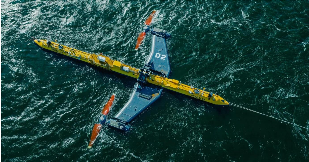
Figure 1. Orbital O2 floating tidal turbine, deployed at the European Marine Energy Center in Orkney, United Kingdom.
